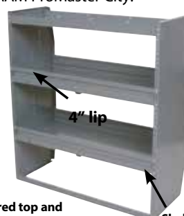
Contoured top and bottom steel end panels maximize aisle space. Shelves adjustable on 1" centers.
